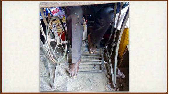
The manual pedals for the machine give him the complete control of the speed of the machine he needs.
